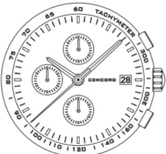
Scale used to measure speed in km/h. Start the chronograph, walk or run exactly 1 km from your point of departure.
